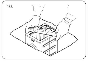
Attach the other end of the ducting into the socket. Use a spirit level to ensure the top of the sockets are level and flush with the ground. Add/remove gravel as required to level.
