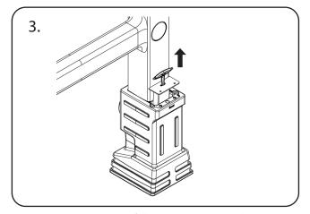
To remove socket wedges, fully insert the Glasdon key into key track, twist slightly to allow the wings of the key to grip the underside of the keyhole and pull the wedges out from each socket.
