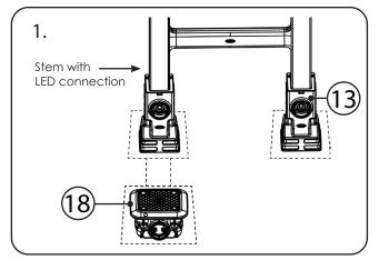
Determine the orientation of the installation. Place the signcarrier into the sockets (ITEM 13), determine where the power supply source is in relation to the installation and mark out the hole locations to suit site requirements and place the Subsafe box (ITEM 18) in place.
