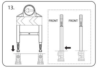
Insert the signcarrier into the sockets and slide forwards to lock into position. The Orbital Chevron should face forwards to match the front facing sockets.
