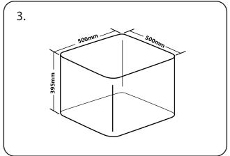
Excavate a hole for the Subsafe to the above dimensions and lay a depth of 50mm of gravel or sand in the base of the hole for drainage. Adapt the excavation to suit cable entry/exit locations and duct requirements. Choose a suitable location to install the Subsafe relative to the signcarrier.
