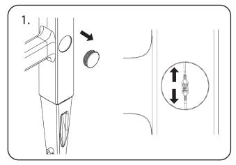
Turn off supply at cut-out (if applicable). Remove the cover cap from the relevant stem and disconnect the snatch plug inside.
