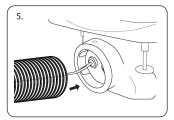
Position the Subsafe box into the hole and orient to suit direction of supply. Feed the power supply cable through the ducting and into the gland, tighten well and connect ducting to unit. We recommend leaving sufficient cable inside the box to enable connection to an IP rated cutout (not supplied).
