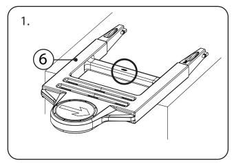
Lay the chevron signcarrier (ITEM 6) down face-up, on a raised, flat surface. So you have access to both sides of the signcarrier, ensure the front of the unit points upwards (Glasdon logo visible).
