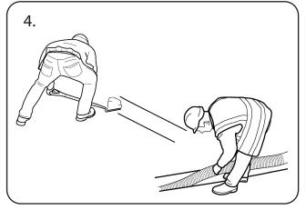
Excavate trenches and lay the required ducting. Between the Subsafe and power supply source and the Subsafe to the Orbital socket, thread the following cables: 1. Power supply from the source to the Subsafe 2. Circuit cabling from the Subsafe to the socket that requires the electricity supply.
