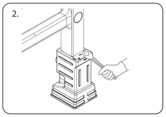
Use a 13mm socket/spanner to untighten the 2x fixing bolts. Remove the fixings.
