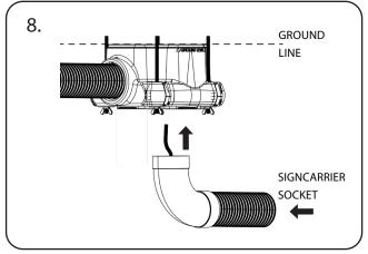
Feed cable from the socket through the ducting to the underside of the Subsafe and thread cable through the gland into the box, tighten well. Leave sufficient cable inside the box to connect to the control circuit housed on the underside of the Subsafe lid.
