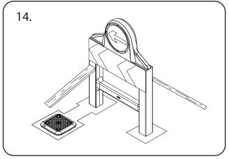
Fill all excavations with concrete. Ensure concrete is flush with the top of the sockets and the fill level on the Subsafe underground box. Smooth the surface and allow concrete to dry for at least 24 hours. We recommend using quick setting concrete (QC 10) and propping up the signcarrier with spare off-cuts whilst the installation sets initially.
