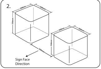
Excavate x2 holes or a trench to the above dimensions for the sockets and lay a depth of 50mm of gravel or sand in the base of the hole for drainage.
