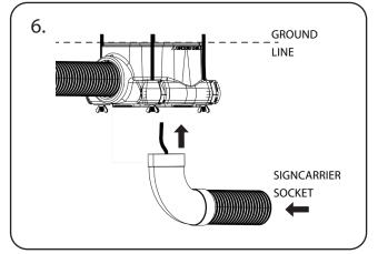
Feed the extension cable through the ducting to the underside of the Subsafe and thread the cable through the gland into the box, tighten well. Leave sufficient cable inside the box to connect to the control circuit housed on the underside of the Subsafe lid.
