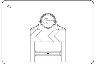
When fitting the standard signboard, ensure the signboard is straight and that the corners of the signboard line up with shoulders on the signcarrier before threading (ITEMS 1 & 2) over each bolt and hand tightening.
