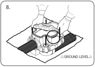
Position the box using a spirit level to ensure that the top is level with the indicator line, to provide a flush installation. Add/remove gravel as required to level.
