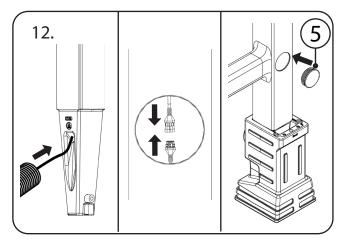
Lay the signcarrier face down with the stems as close to the sockets as possible. Feed the cable from the socket up into the left hand signcarrier stem through the small access hole until it is visible through the access hole to the rear of the signcarrier. Connect the two halves of the snatch plug together. Position the stem access plug (ITEM 5) over the hole and push in.
