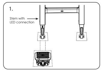
Determine the orientation of the installation. Determine where the power supply source is in relation to the installation and mark out the hole locations to suit site requirements for the Signcarrier and Subsafe.
