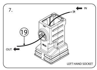
Thread the extension cable through the left hand socket and out of the connection point. We recommend attaching a piece of string around the end of the cable end to prevent it from falling through. Ensure a minimum of 2m is left on the 'IN' end to enable connection to the LED connection cable.
