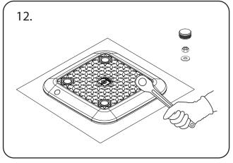
Turn on the power (i.e. via cut-out) and the signcarriers round signface will illuminate. Place the lid onto the Subsafe and position (ITEMS 16 & 17) into each of the Subsafe's fixings. Tighten fully using a 13mm socket/spanner. Insert a cover cap over each fixing (ITEM 15).
