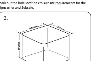
Excavate a hole for the Subsafe to the above dimensions and lay a depth of 50mm of gravel or sand in the base of the hole for drainage. Choose a suitable location to install the Subsafe relative to the signcarrier to suit site requirements.
