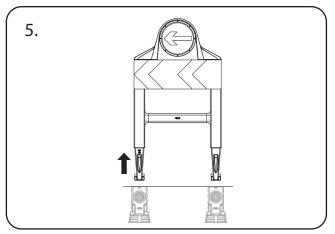
Lift the signcarrier out from the sockets. Take care when removing the cable and snatch plug from the stem before moving the signcarrier away.
