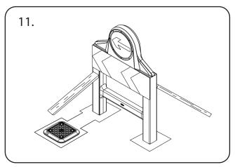
Fill all excavated holes with concrete. Ensure concrete is flush with the ground level indicator of the Subsafe and the top of the stems. Smooth the surface and allow concrete to dry for at least 24 hours. We recommend using quick setting concrete (QC 10) and propping up the signcarrier with spare off-cuts whilst it sets.
