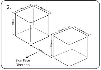
Excavate x2 holes or a trench to the above dimensions for the extended bases and lay a depth of 50mm of gravel or sand in the base of the hole for drainage.
