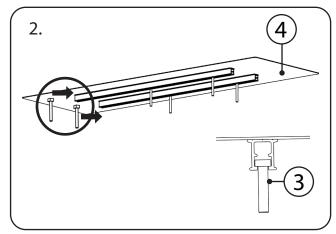
Slide the x6 square headed bolts (ITEM 3) along the rails on the back of the signboard (ITEM 4), using x3 bolts per rail.
