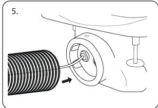
Position the Subsafe box into the hole and orient to suit direction of supply. Feed the power supply cable through the ducting and into the gland, tighten well using a 13mm socket/spanner and connect ducting end to unit. We recommend leaving sufficient cable inside the box to enable connection to an IP rated cutout (not supplied).
