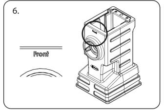
Place the sockets into the deeper excavations. Ensure the sockets are orientated correctly. The sockets should be installed with the word 'FRONT' facing oncoming traffic.
