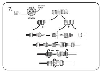
Thread one side of the IP68 rated plug onto the end of the extension cable and the other end onto the 'supply out' cable from the housed control circuit as shown above. Ensure (BLACK & RED) cables are connected to the correct pins. Connect the plugs and twist to seal.
