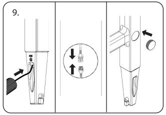
Lay the signcarrier face down with the stems as close to the excavation as possible. Feed the other end of the extension cable into the left hand signcarrier stem through the small access hole until it is visible through the access hole to the rear of the signcarrier. Connect the two halves of the snatch plug together. Position the stem access plug (ITEM 5) over the hole and push in.
