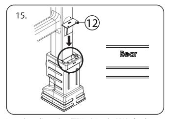
Insert the socket wedges (ITEM 12) into the REAR of each socket. Position (ITEMS 9 & 10) into each of the sockets' fixing holes and tighten fully using a 13mm socket/spanner.
