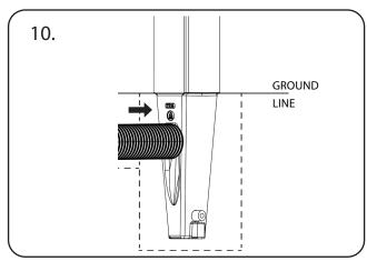
Place the signcarrier into the hole, position the ducting up to the left hand stem. Add / remove gravel as required to help position the signcarrier at the correct height. Use a spirit level to ensure the top of the signboard is level with the ground and the signcarrier is vertical.
