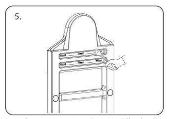
Return the signcarrier to its' up-right position. Fully tighten the signboard fixings using a 13mm socket.
