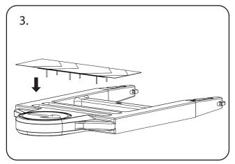
Lower the signboard down on top of the signcarrier. Ensure the rails on the back of the signboard line up with the rail slots on the signcarrier and that the x3 bolts are inserted into each bolt slot on the signcarrier for most secure installation.
