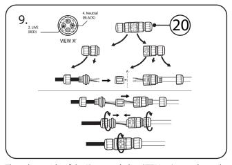
Thread one side of the IP68 rated plug (ITEM 20) onto the end of the extension cable and the other end onto the 'supply out' cable from the housed control circuit as shown above. Ensure (BLACK & RED) cables are connected to the correct pins. Connect the plugs and twist to seal.
